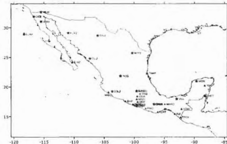
Fig. 2. The network of continuous GPS receivers of Institute of Geophysics of UNAM (red triangles) and National INEGI network (blue stars). (For interpretation of the references to colour in this figure legend, the reader is referred to the web version of this article.)
